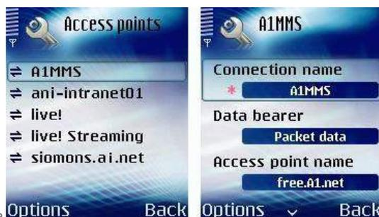
Figure 4. Configuring APN on device
