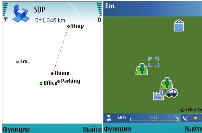
SDP allows user to select landmarks from the database to display them on the screen and to calculate the distance between them. Latitude and longitude - these coordinates are used for defining the location of the point on the sphere surface. For displaying the landmarks on the rectangular screen, we can provide the value of latitude as Y, and longitude as X. This approach allows to display data enough exactly, if the landmarks are located not very far apart.
